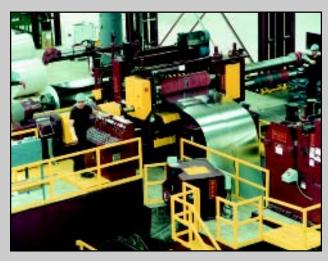
Slitter Design: The Slitter is a quick-change "Turret" equipped with two 10.000" slitter heads. The Turret slitter is manufactured to precision machine tool tolerances and utilizes "shimless" slitter tooling that is lapped to within .000040", giving Baldwin the ability to produce precision tolerance slit coils. With clear access to the arbors during set-up (making re-
