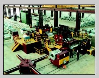
**Control:** Operator friendly line controls are designed for ease of operation and visibility. The main operator console is elevated, giving the line operator an excellent view of the coil from entry to exit. Remote control stations are installed at both ends of the line for fast and safe coil loading and unloading.
