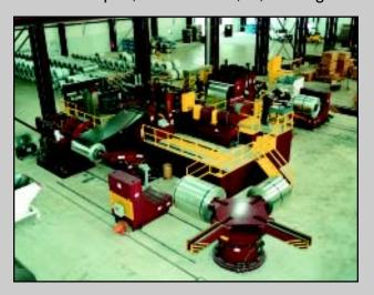
to process coated and bare cold rolled, and hot rolled pickled coils in sizes up to 80,000# x 72" wide, with coil diameters to 84". The line has the ability to slit mild and high strength steel coils in gauges ranging from .010" through 3/16" at line speeds up to 1,000 FPM.
