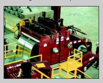
incorporates "slide-out" replaceable pads that can be exchanged in about 30 seconds. The roll tensioner utilizes tension rolls with a unique "non-sliced" surface that eliminates the "smut" that diced or sliced rolls apply to the strip surface. Two sets of strip guides are included in the tensioning equipment to separate and guide the strips. A quick-change speed load device allows for "off-line" set-up of the guides and an exchange that takes about a minute.
