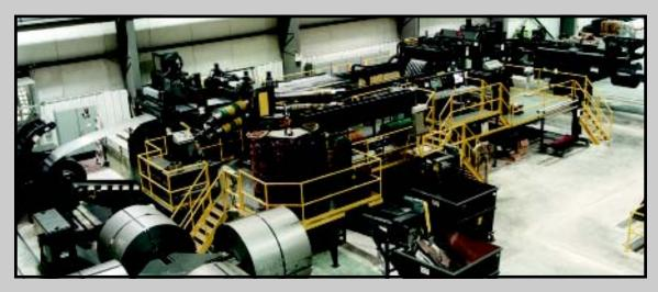
The new slitting line is capable of processing hot band, hot rolled pickled, and cold rolled high strength coils in gauges from .010" through .250". The line will handle 80,000# x 72" wide coils with coil diameters up to 84". 850 line horsepower is utilized to process lighter gauges in the "free loop" mode at 1,500 FPM. Heavier gauges are processed in either "push-pull" or "tight line" modes at 500 FPM.
