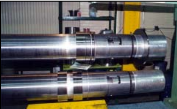
Locking fingers retracted for re-tooling
