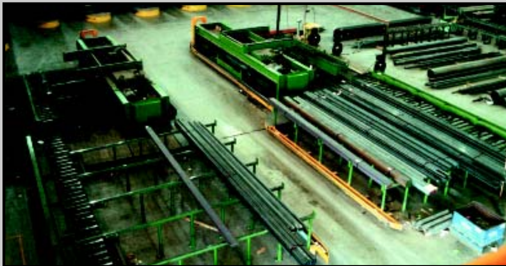
Two Braner/Loopco Long Products Bundling Systems operating in a Midwestern metal distribution plant.
