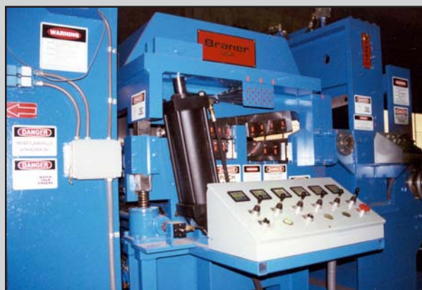
1/4"-.015" Shape Correction Leveler
