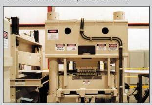
The Leveler controls feature full automatic Leveler set-up based upon gauge and yield strength inputs, a computer memory that recalls previous Leveler set-up parameters (saving set-up time when running partial coil orders), and a calibration mode that automatically calibrates the Leveler after roll grinding or periodic maintenance.
