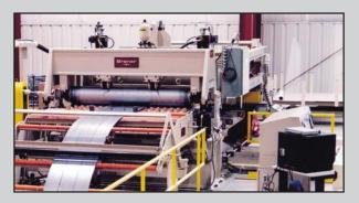
The electronic motion control receives feed roll position data from an electronic encoder, and the position information is instantly transformed into accelerate, decelerate, and full stop commands based upon the feed length. The motion-control system automatically computes the ideal production speed based upon the part length entered into the operator data panel. An adjustable acceleration/deceleration control is provided to compensate for various material surface conditions.
