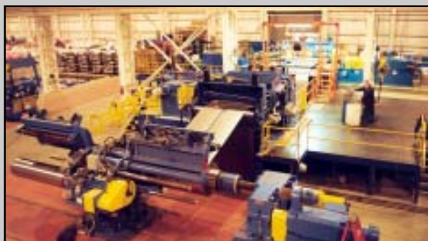
76" Slitting Line (Inspection Station in background)
