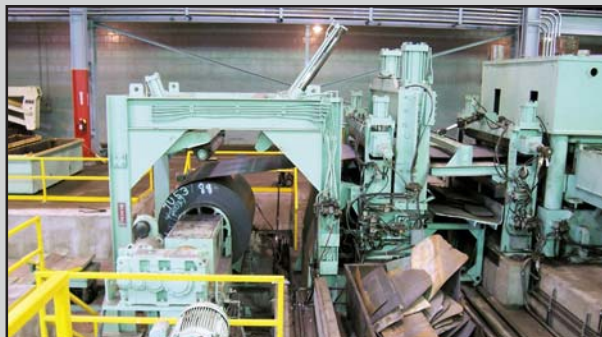
Cone Uncoiler, Hold-Down, Set-Breaker Roll, & Crop Shear
