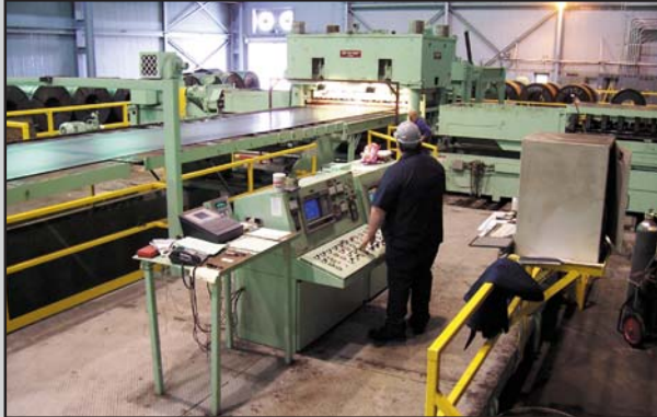
Cassette Leveler Producing Panel Flat Hot Band Sheet
