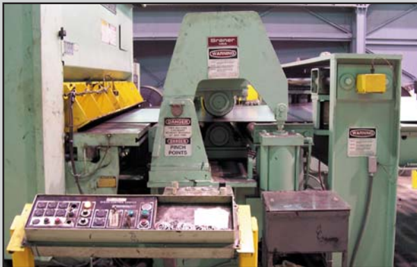
Right to Left: Squaring Guides, Servo Roll Feed, & Hydraulic Shear
