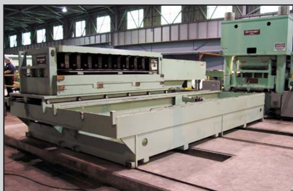
3.000" Cassette Stored on the Injector Cart. 5.500" Cassette is Installed in the Leveler
