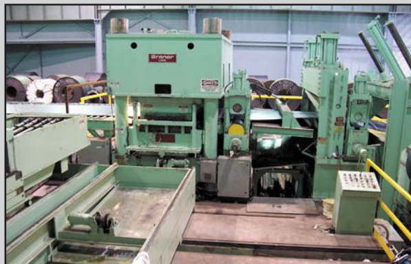
Massive 4-Post x 500HP Hydraulic Cassette Leveler
