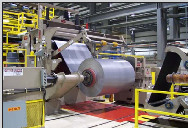
Automatic Tracking Recoiler with Over and Under Rewind Capability
