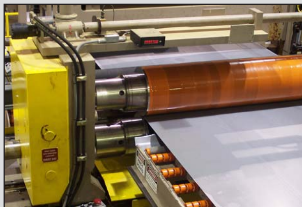
3 Head Turret Head™ Slitter w/Pushbutton Tooling Lock-Up
