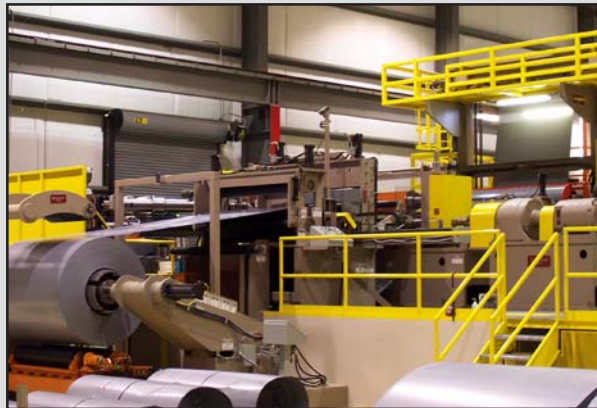
250 HP-DC Loop-Control/Drag Generator Uncoiler
