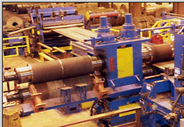
15" x 84" x 400HP Turret Head™ Slitter
