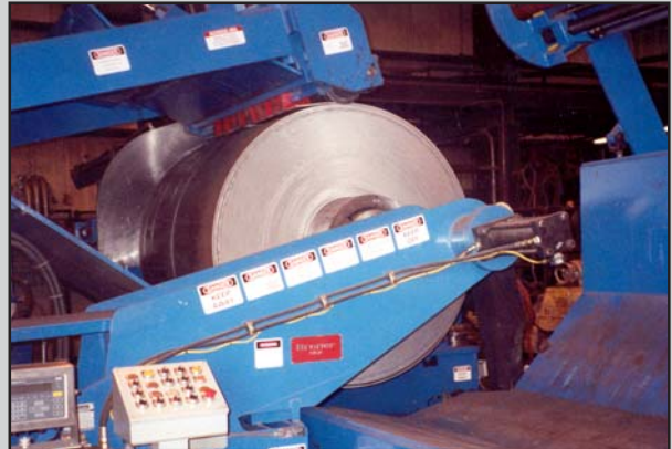
90,000# x 84" x 400HP Recoiler w/Outboard
