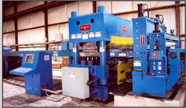
1.750" x 17-Roll x 9-Flight x 5-Hi Hydraulic Leveler
