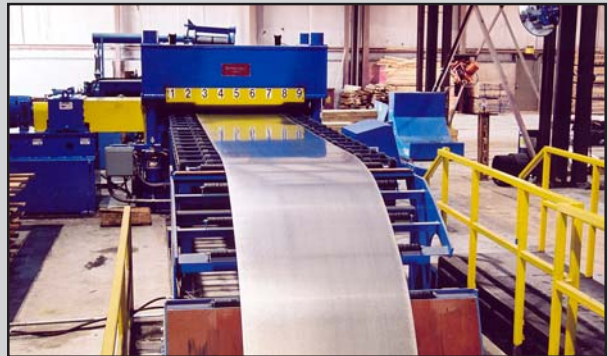
Flatness Inspection Table & Loop Quadrant
