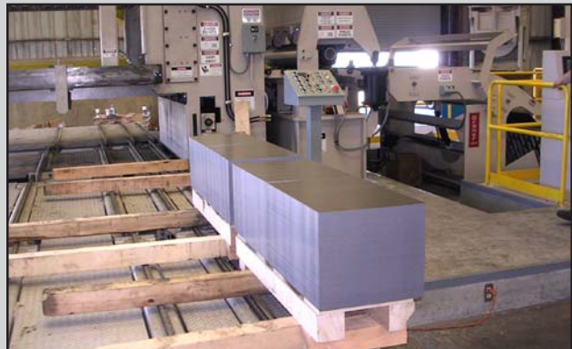
Programmable Stacker Produces Solid-Block Multi-Blank Stacks
