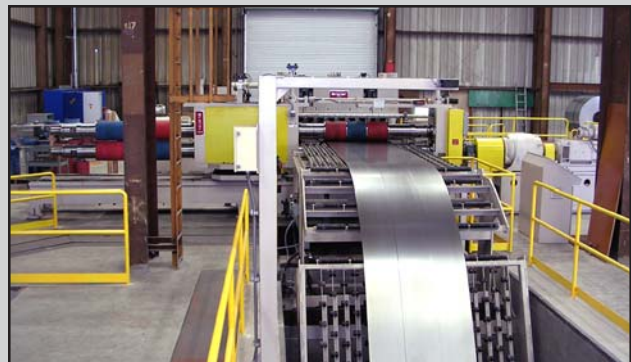
Quick-Change "Pushbutton Tooling Lock-Up" Turret Head™ Multi-Blanking Slitter with Off-Line Set-Up Ready to Exchange
