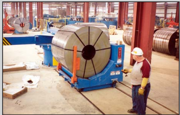
"Wireless" controls are installed on both Entry & Exit Coil Cars. Freedom of movement allows operators to safely control Coil Cars from 10' away.
