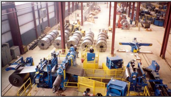
High-production 60,000# x 60" x 1/4" Single-Loop Turret Head™ Slitting Line conserves floor space.
