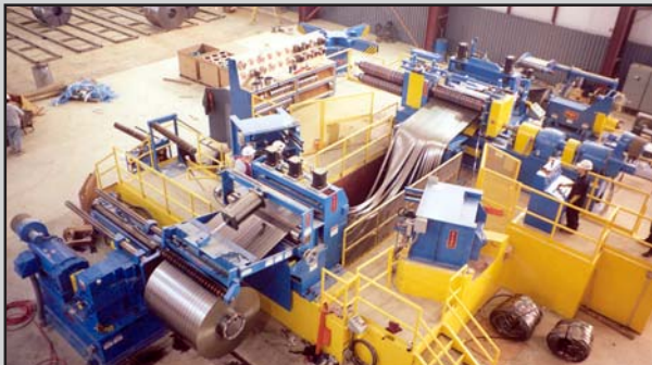
The entire slitting line from end to end is within clear view of the operator, important for safety and operating efficiency.
