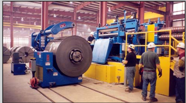
"Wireless" controls are installed on both Entry & Exit Coil Cars. Freedom of movement allows operators to safely control Coil Cars from 10' away.
