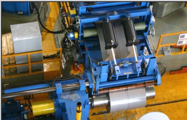
Rigid Overarm Separator with “swing-out” quick-change tooling arbor and tail hold-downs.
