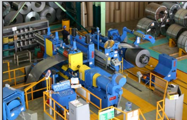
Entry end view shows compact Uncoiler to Slitter spacing.
