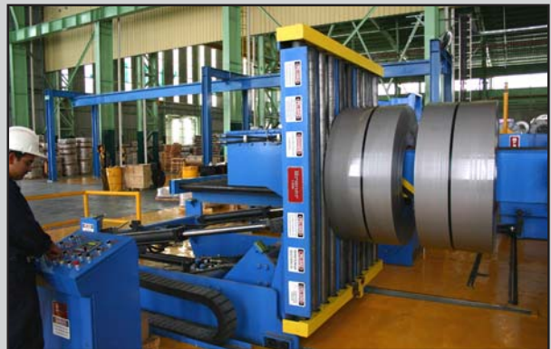
Fully automatic “operatorless” Programmable Slit Coil Downender.
