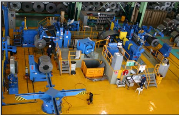
25-ton x 60" x 1/4" Single-Loop Turret Head™ Slitting Line. Notice the entire slitting line is within clear view from the main operator station.
