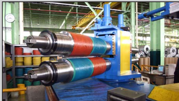
Completely exposed and accessible arbors cuts re-tooling time and strain. No housings or bases obstruct the removal or installation of the slitter tooling. Head are exchanged in less than 2-minutes
