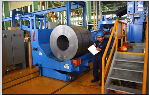
Tight straight wall slit coils are quickly unloaded from the Recoiler by Coil Car with easy to use “wireless” operator controls.
