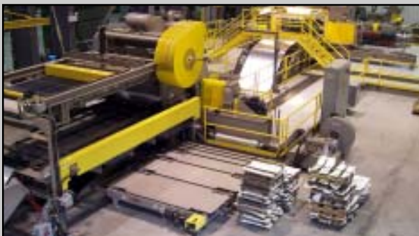
72" Multi-Blanking Line Exit End View
