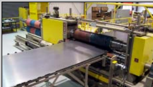
Quick-Change "Pushbutton Tooling Lock-Up" Turret Head™ Multi-Blanking Slitter with Next Set-Up Ready to Go
