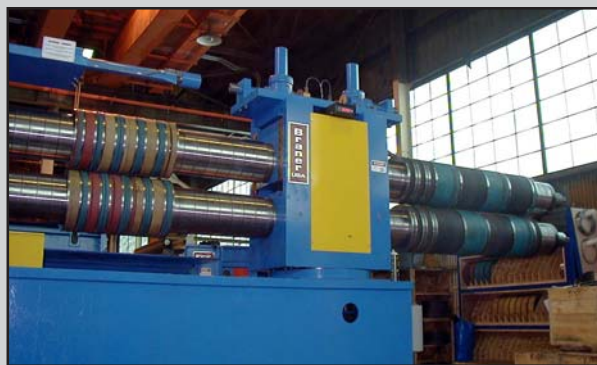
Completely exposed and accessible arbors minimize tooling time. Heads are exchanged in less than 2 minutes.
