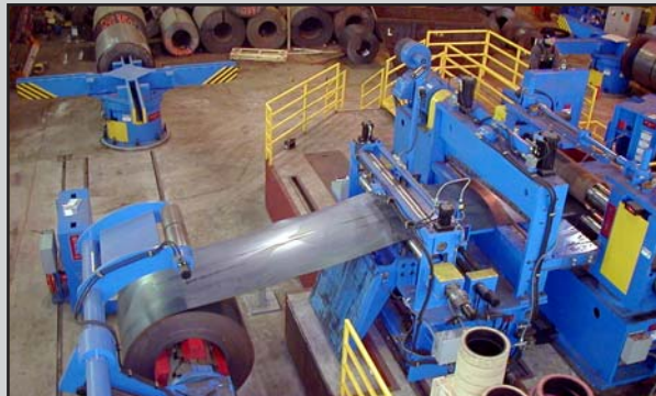
Strip runs over the Pass Line Roll to prevent surface marking. Lightweight "Red" Fillers handle 28"-32" ID master coils
