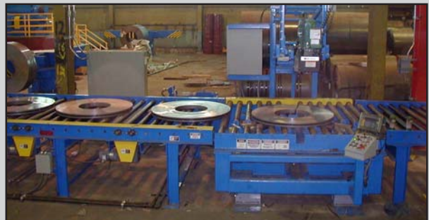
Coiltech Semi-Automatic Strapping Machine and automatically controlled Power Conveyor feed the stacking equipment.
