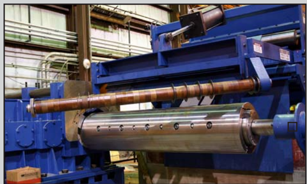
Swing-out Overarm arbor exchanges tooling in minutes.
