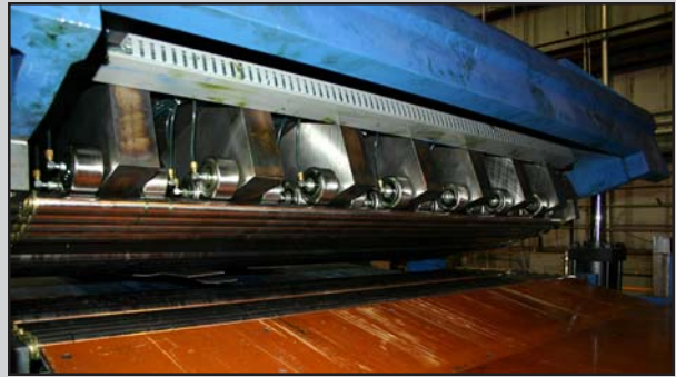
View of upper work rolls and back-up flights
