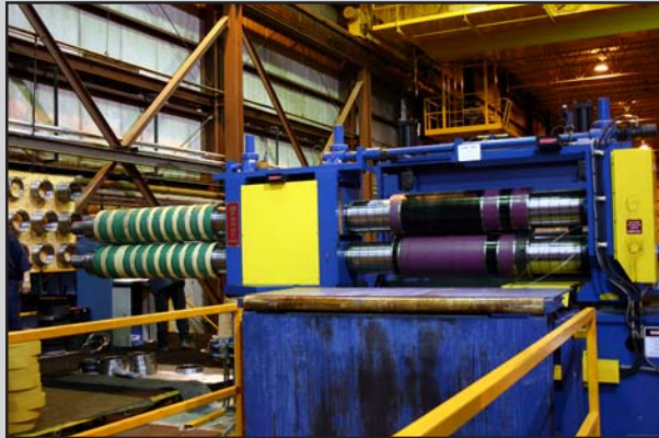
Completely exposed and accessible arbors reduces set-up time
