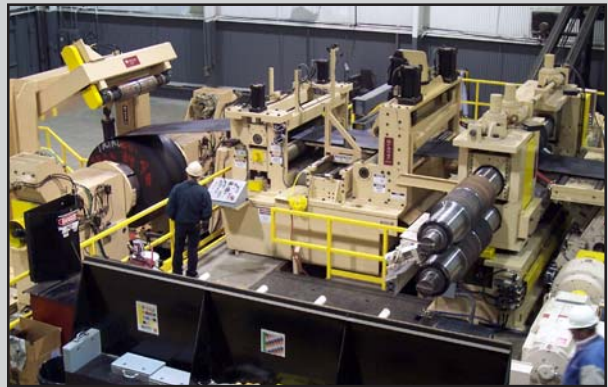
View of Uncoiler, Hold-Down, Straightener, Guides, & Shear ahead of the Turret Slitter
