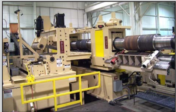
Open and accessible arbors cuts re-tooling time. There are no housings or bases that interfere with re-tooling
