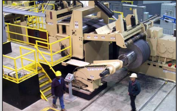
Strip Tensioner, Overarm, and Recoiler
