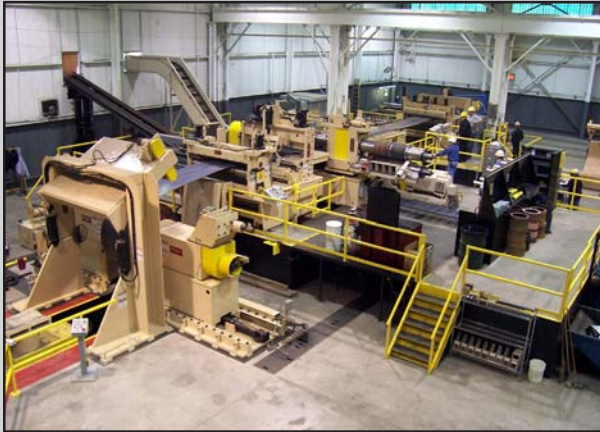
80,000# x 72" x 3/8" Single-Loop Turret Head™ Slitting Line. Notice Crop Shear & Chopper conveyors deliver scrap to outdoor scrap boxes.
