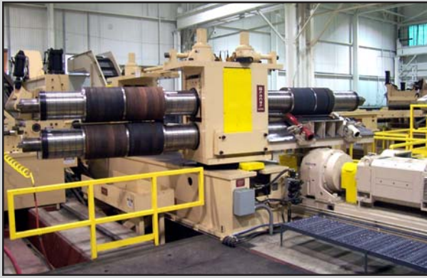
12" x 72" Turret Head™ Slitter can exchange heads in less than 2-minutes. Scrap guides are pre-set with the Slitter set-up.
