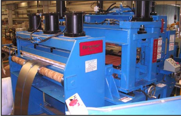
Quick-change Pad and Acu-Trak Tensioners generate enormous rewind tension
