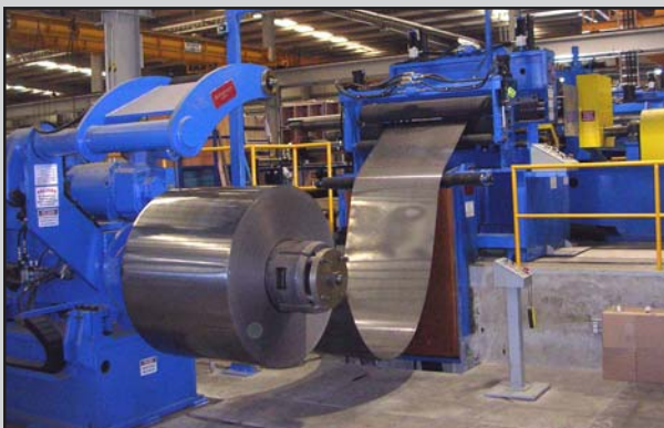
Driven Loop-Control Uncoiler allows “tension-free” slitting for improved thin-gauge surface-critical coil quality
