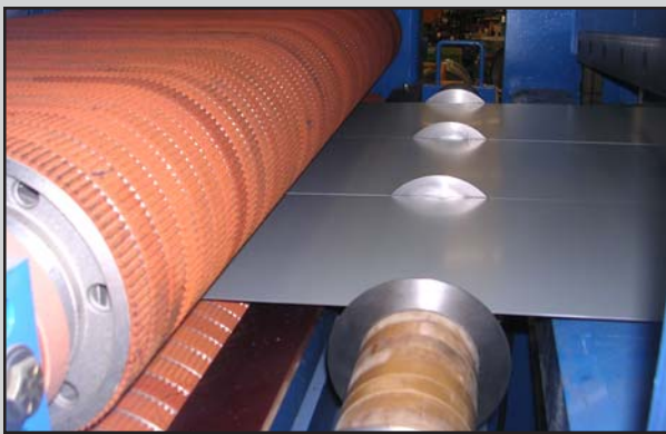
Acu-Trak Tensioner employ high friction non-marking belts to generate rewind tension for surface-critical materials
