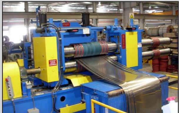
Completely exposed and accessible arbors re-tool quickly. No frames or bases obstruct the removal or installation of the slitter tooling. Head are exchanged in less than 2-minutes.
