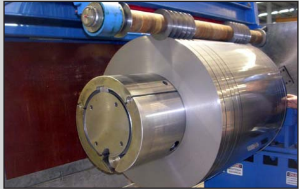
2" thick forged heat-treated Recoiler steel drum with 3" steel gripper bar
