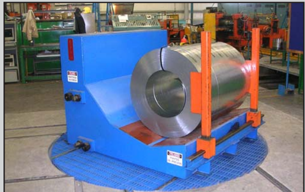
"Wireless" controls are installed on both Entry & Exit Coil Cars. A Turntable redirects the Car travel direction.
