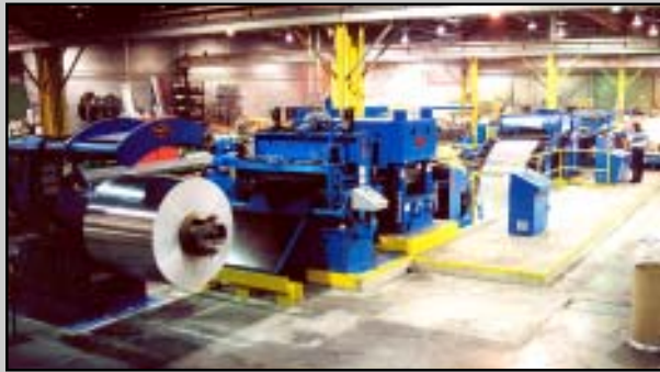
Precision Hydraulic Leveler-Servo-Feed Steel & Aluminum CTL Line
