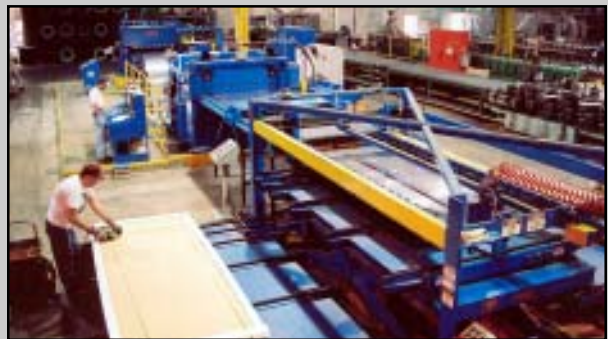
Exit End View of the ATAS Surface-Critical CTL Line
