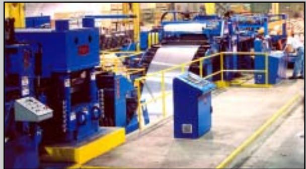
Side view of the ATAS CTL Line. Coil mechanical properties are entered into the "touch-screen" computer terminal console (center). A Laminator applies protective PVC film ahead of the Shear.
