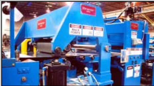
Hi-Cyclic Rate Precision Electronic AC Servo-Feed Processing Surface-Critical Aluminum
