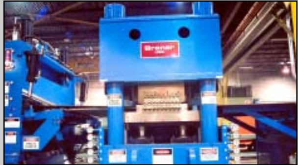
Precision Microprocessor Controlled Hydraulic Leveler
