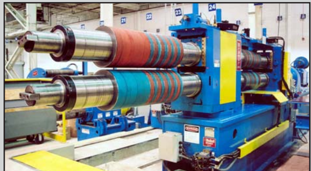
Turret Head™ Slitter changes from one order to the next in about one-minute
