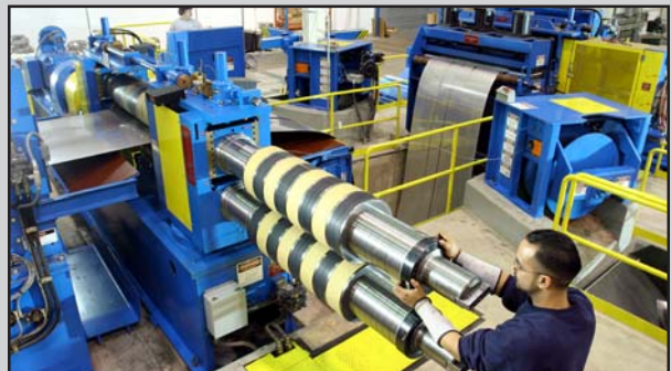
A Turret Head™ Slitter is more rigid and precise than any other multi-head slitter design, and because the arbors are easily accessed with no obstructions, re-tooling and order change is accomplished faster than with any other slitter head design
