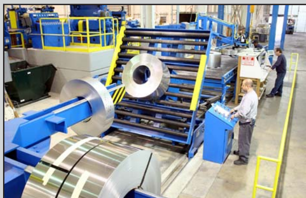
Downender automatically "travels and picks" coils off the Turnstile arm. Various coil sizes are programmed into a PLC keypad.
