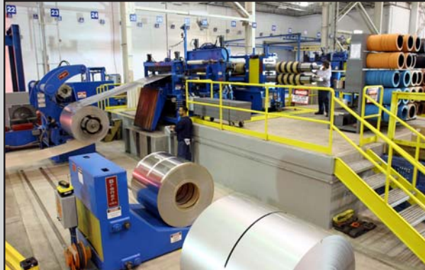
Hi-production 40,000# x 60" Turret Head™ Slitting Line processing a paper interleaved 304 stainless coil. A "wireless" control Coil Car loads the Slitting Line
