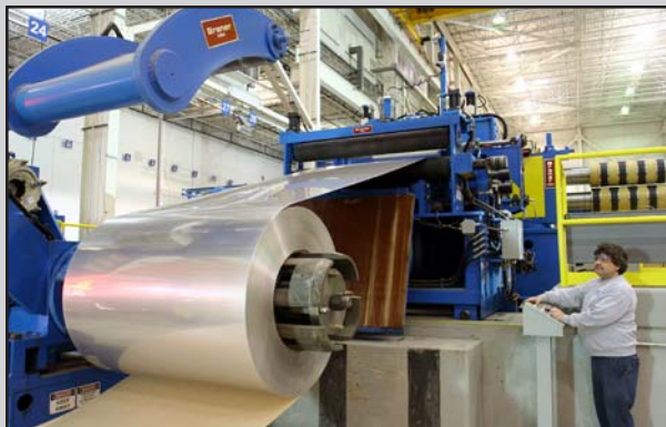
Hi-Pass Line eliminates top-side strip scuffing and reverse strip bending
