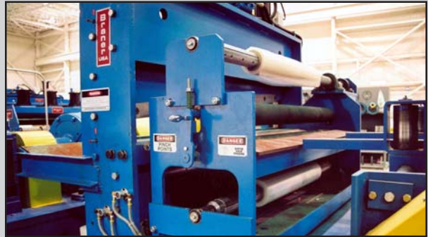
Top and bottom PVC Laminator with expandable shafts and quick-open laminating rolls
