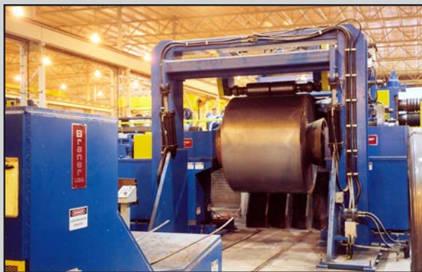
DC Motor Cone Uncoiler and Free-Standing Coil Hold-Down
