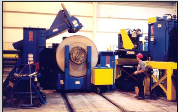
Coil Unloading Car with Wireless Controls
