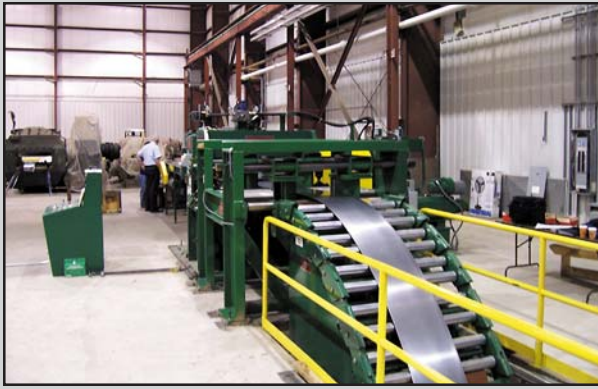
Flat Strip Supported on the Exit Quadrant and Entering the Strip Guides
