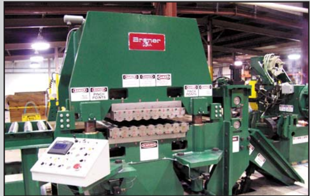
17-Roll Backed-Up Straightener Produces Panel Flat Hi-Strength Strip
