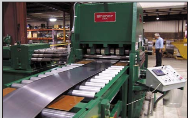
Panel Flat Hi-Strength Strip Emerging from the Backed-Up Straightener. Automatic Roll Gap Controls Speeds the Set-Up Process
