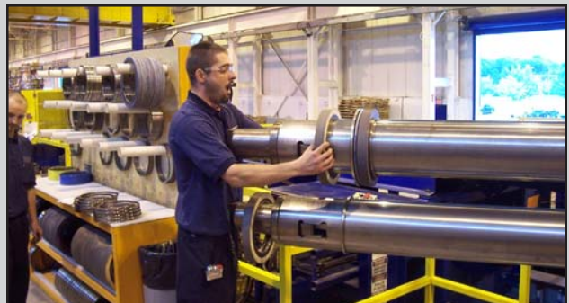
Turret Head™ Slitter arbors are easily accessible with no obstructions so re-tooling is accomplished faster with less set-up fatigue than with any other slitter head design.
