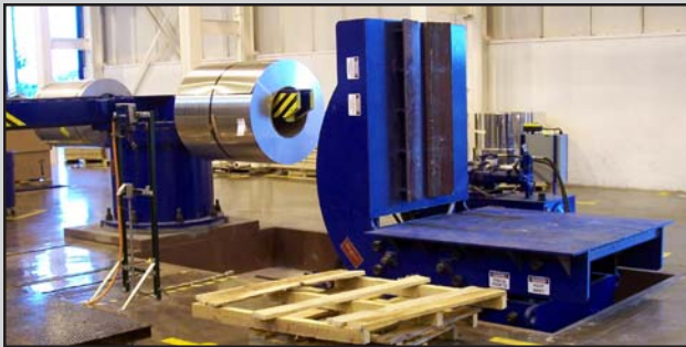
Coil Car-Tipper upends palletized coils and loads onto a 4-Arm Entry Storage Horn
