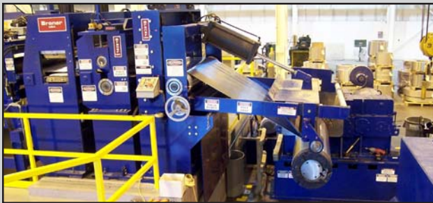
Tension Pad and Non-Marking Tension Rolls can be employed in tandem or engaged independently.
