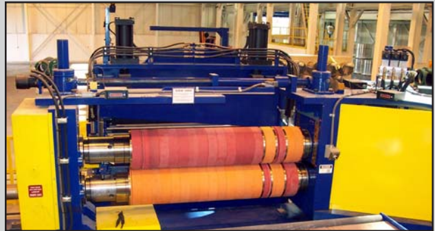
Pushbutton tooling lock-up Turret Head™ Slitter exchanges Slitter heads in about one-minute
