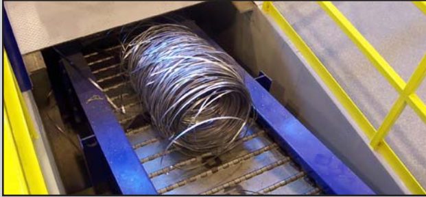
A steel belt conveyor carries scrap bundles to a scrap container.
