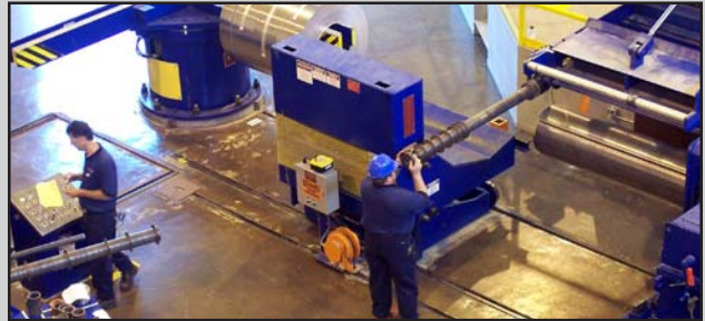
A swing-out Speed Load Overarm arbor allows for quick exchange of pre-tooled separator arbors without lifting
