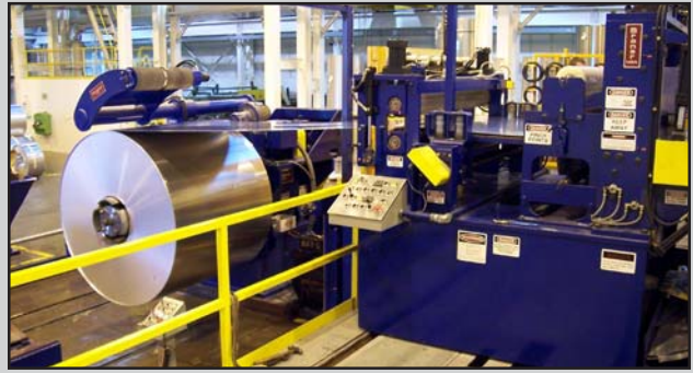
DC Loop Control Uncoiler operates in single and double-loop operating modes. The Slitter Entry Unit is equipped with power adjusted Side Guides, Automatic Edge Guide, PVC Laminator, and an Entry Crop Shear
