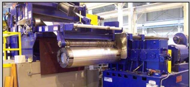
250 HP x 16" ID Recoiler with 20" One-Minute Speed-Load Fillers
