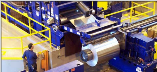
Exit Unit supports the Exit Shear, Side Adjust Overarm, Pass Line Roll, and Paper Interleaver
