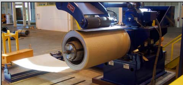
Interleaved Paper Winder efficiently handles interleaved paper
