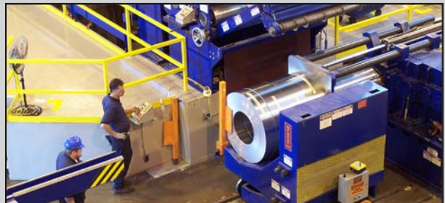
Wireless Coil Car control allows Car operation from a safe distance.
