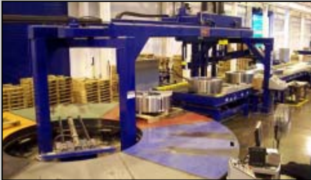
Second coil is centered in the Stacker awaiting transport to the stacking station
