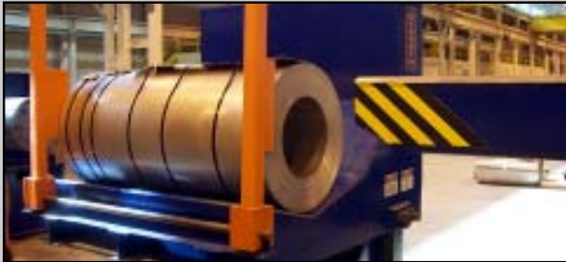
Wireless control Coil Car transferring slit coils from the Slitting Line to a 4-Arm Turnstile
