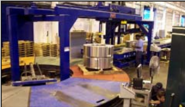
Two coil package completed at the stacking station
