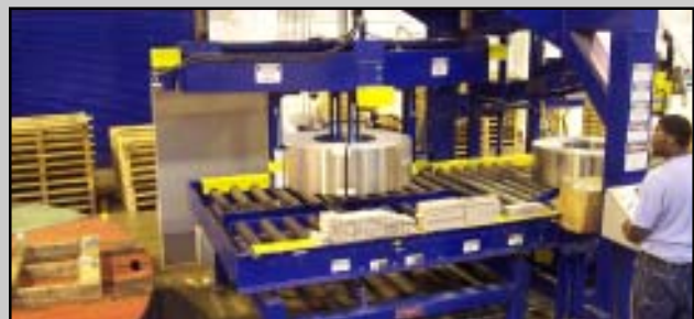
Coil is centered in the Stacker and secured from the ID and OD for transport to the stacking station
