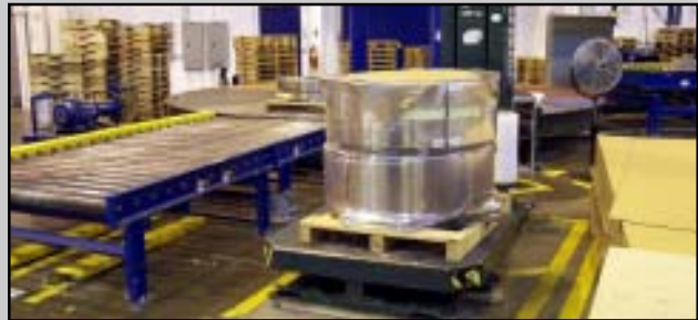
Free standing Stretch Wrapper applies protective wrap for shipping
