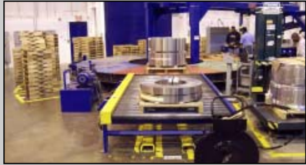
Two coil package positioned for discharge from the Turntable
