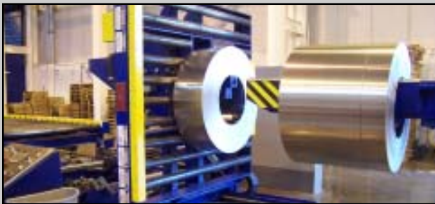
Programmable Slit Coil Downender automatically separates and downends coils
