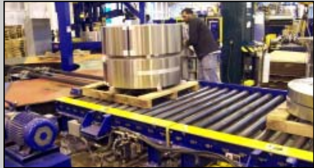
Completed package discharged from the Turntable onto the Weigh Station
