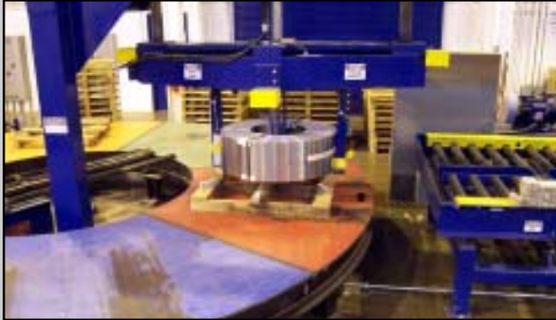
Coil deposited onto pallet at the Turntable stacking station
