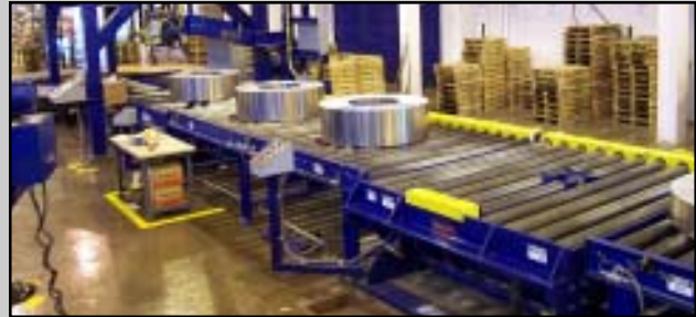
Staging Conveyor automatically advances coils to the Strapping Machine
