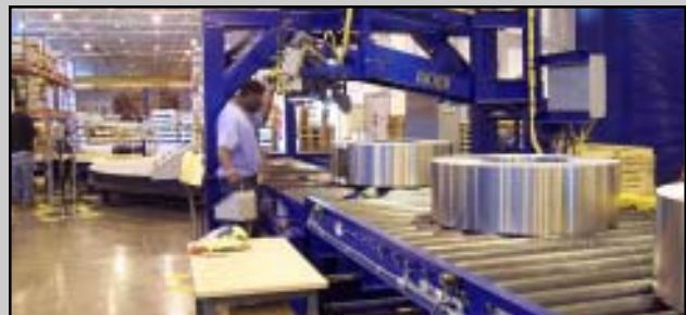
Semi-Automatic Strapping Machine applies radial straps
