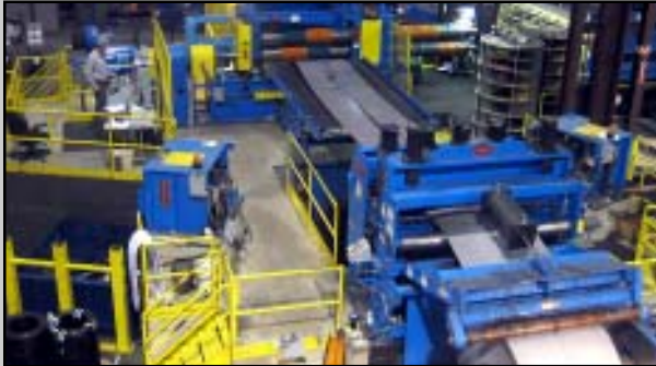
60,000# x 72" x 1/4" Single-Loop Turret Head™ Slitting Line
