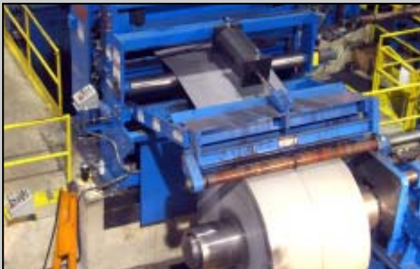
Exit end equipment generates strip tension; crops coil tails; and rigidly supports the Overarm Separator and Threading Funnel.
