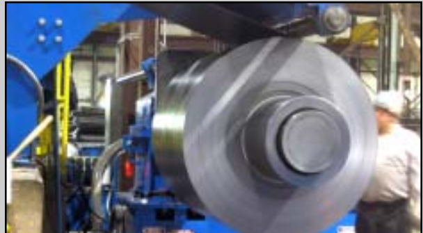
Massive 250-HP 2-ratio Recoiler has a 14" diameter main shaft
