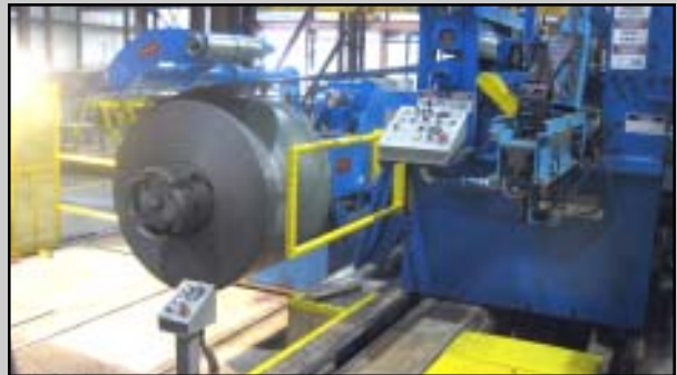
Unique Entry Coil Prep Station combines entry coil threading and guiding equipment into a single compact machine that speeds coil loading and threading
