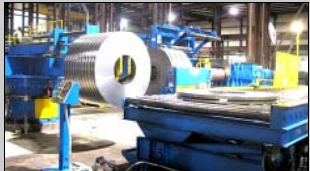
A Slit Coil Downender removes coils from the 4-Arm Exit Turnstile and feeds the coils to the Strapper and Coil Stacker.
