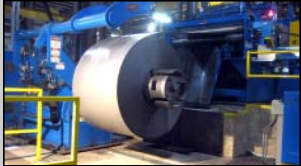
Coil are processed with no reverse strip bending against the natural coil-set, which eliminates equipment induced coil-breaks
