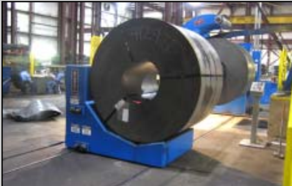
60,000# coils are staged on an Entry Turnstile and loaded by Floor Level Coil Car
