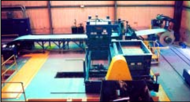
60,000# x 72" x 1/4" Cassette Leveler-Servo-Feed-DC Shear CTL Line
