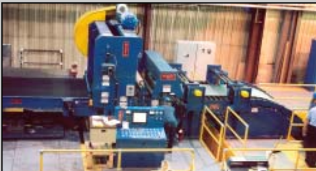
Loop Quads and Side Guides square the strip into the Servo-Feed and DC Shear
