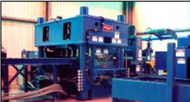
Precision Microprocessor Controlled Hydraulic Cassette Leveler
