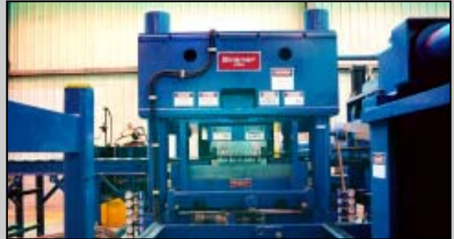
4-Post Cassette Leveler with 1,500" Cassette Installed
