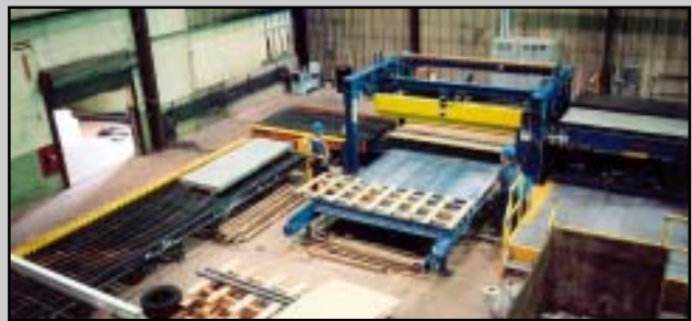
Exit End View of Macsteel 72" x 1/4" CTL Line
