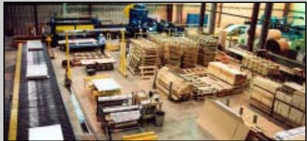
Inspection-Reject Belt, Sheet Stacker, and Programmable Pallet Injector
