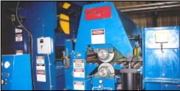
Hi-Cyclic Rate Electronic AC Servo-Feed with "pull-back" sequence avoids Shear blade scuffing.
