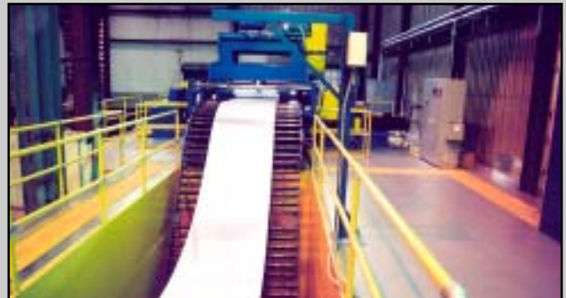
Servo-Feed draws leveled strip from a free-loop between the Cassette Leveler and Servo-Feed
