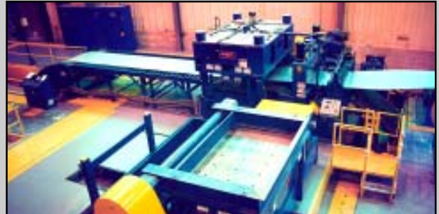
1,500" Cassette leveling .024" embossed aluminum coil. The 3,000" Cassette is stored on the Injector Car ready to level .250"-.060" coil.
