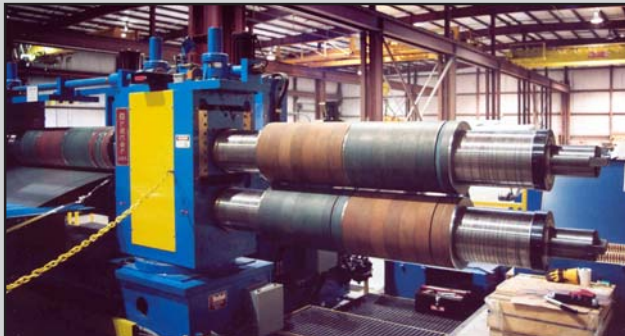
Turret Head™ Slitters can be re-tooled faster with less fatigue than with any other quick change slitter because no base or frames impede access to the arbors
