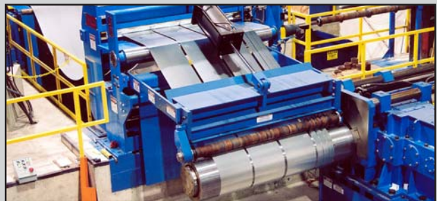
Compact Hi Pass Line provides superb slit strip tracking regardless of strip width, gauge, and number of cuts.
