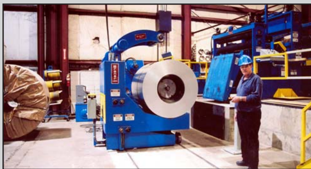
Coil Loading Car is equipped with a unique "wireless" control that allows the operator excellent mobility while maintaining a safe distance from the Car and the coil.
