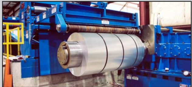
Massive 250-HP 2-ratio Recoiler has a 14" diameter main shaft and a full-face ground surface coil pushoff
