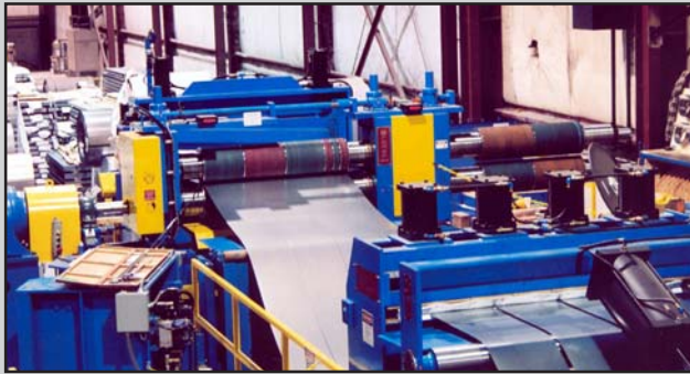
Turret Head™ Slitters set-up faster, change heads faster, and occupy less floor space than any other Slitter design.
