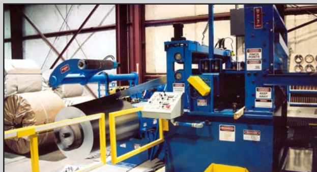
Entry Coil Prep Station combines entry coil threading and guiding equipment into a single compact machine that speeds coil threading and improves strip tracking
