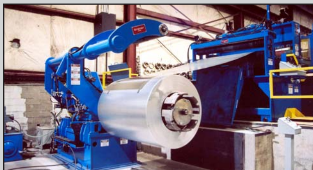
Coils are processed with no reverse strip bending against the natural coil-set, which eliminates equipment induced coil-breaks. Hi pass line also provides excellent strip tracking and preserves floor space
