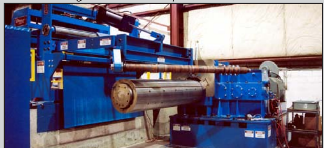
Unique swing-out Overarm arbor allows pre-tooled Overarm arbor exchange to be accomplished in minutes.
