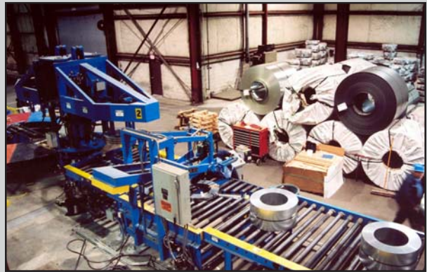
Narrow coil being strapped while wide coils await advancing into the Strapper
