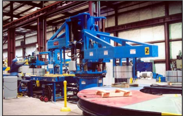
Turret Stacker stacking a wide slit coil onto a pallet located on the Turntable
