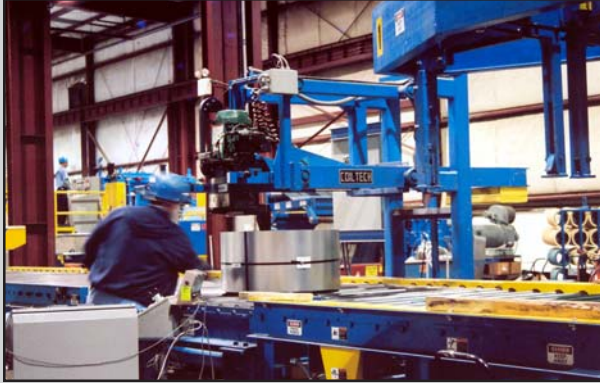
Strapping Machine manipulates the coil and applies radial straps in a semi-automatic manner
