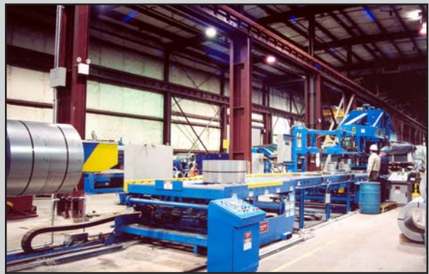
Staging Conveyor automatically advances coils to the Strapping Machine
