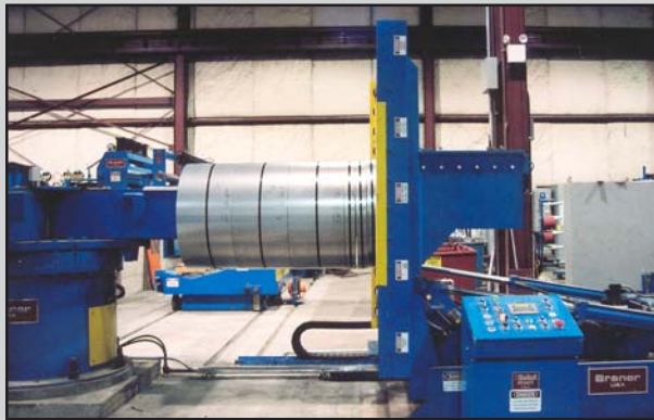
Programmable Slit Coil Downender automatically travels to the 4-Arm, "picks" individual slit coils off the 4-Arm, and downends the coils for strapping & stacking
