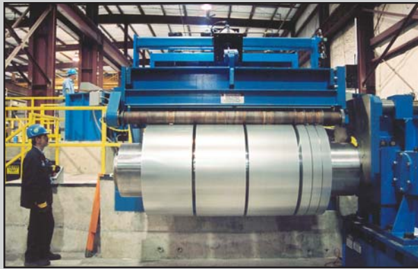
Slit coils generated from the 72" Braner/Loopco Slitting Line will be packaged on Lafayette's Automatic Slit Coil Packaging Line.
