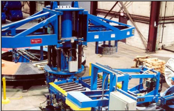
Turret Stacker carries a "batch" of coils to the Turntable while the opposite empty head travels back to retrieve a coil from the centering table. Double stacking heads with "multi-grab" programming makes the Turret Stacker extremely efficient.
