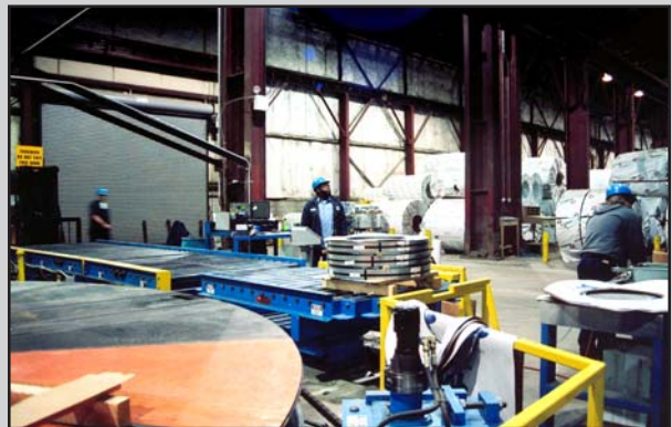
Rotary Pallet Bander speeds strapping coils to the pallet.
