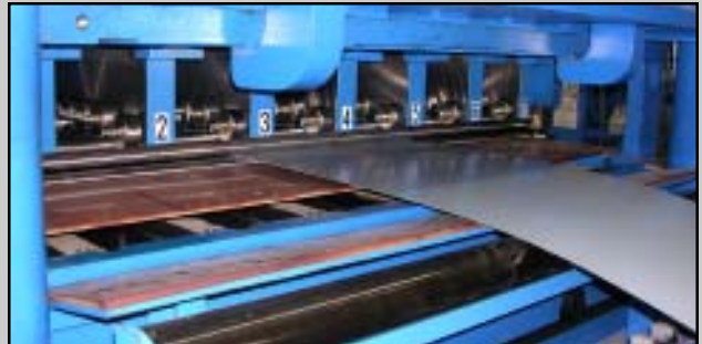
1.250" x 17-Roll x 5-Hi Cassette Leveling .018" Side-Trimmed Electro Galvanized Coil
