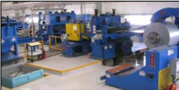
Entry Section allows coils to be unwound from top or bottom
