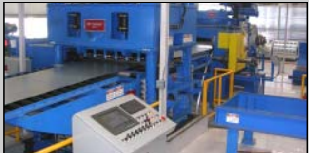
Cassette Leveler employs multiple Cassettes for processing a .016"-.125" gauge range
