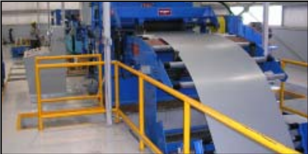
Precision Electronic AC Servo-Feed Processing Surface-Critical Strip
