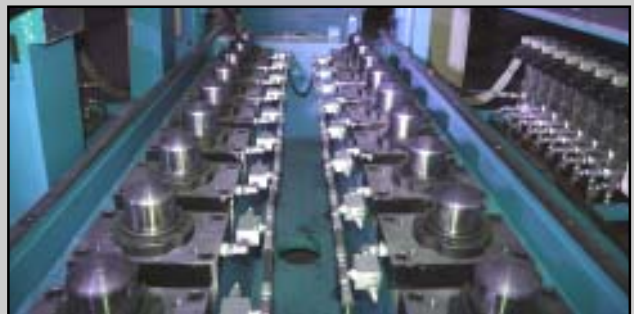
View inside a 4-Post Cassette Leveler Frame shows linear transducer controlled hydraulic cylinders that adjust Cassette back-up flights
