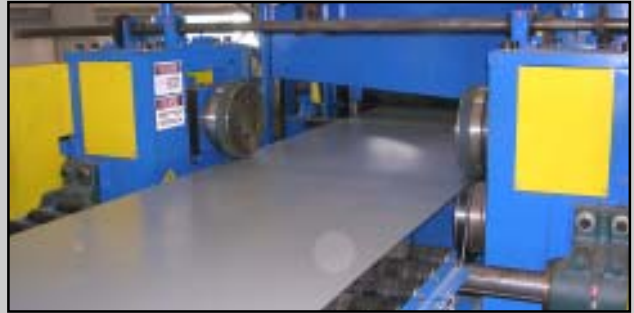
Stub-Arbor Side Trimmer generates precision width strip nance, and improved "up-time" because roll cleaning & maintenance is accomplished while the Leveler remains in operation with another Cassette.
