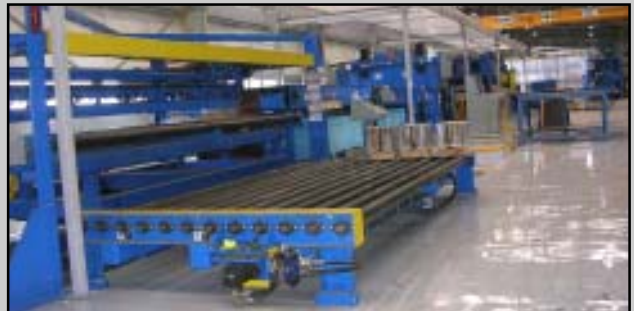
Automatic Pneumatic "Flipper" Sheet Stacker & Runout Conveyor Productivity and bullet-proof reliability made JFE Shoji's choice of a Braner/Loopco Cut-to-Length Line a "no-brainer".
