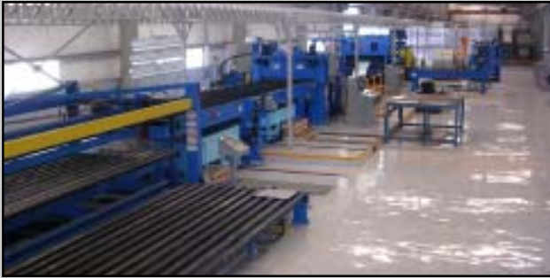
60" x .125"/.016" Cassette Leveler/Servo Feed CTL/Blanking Line
