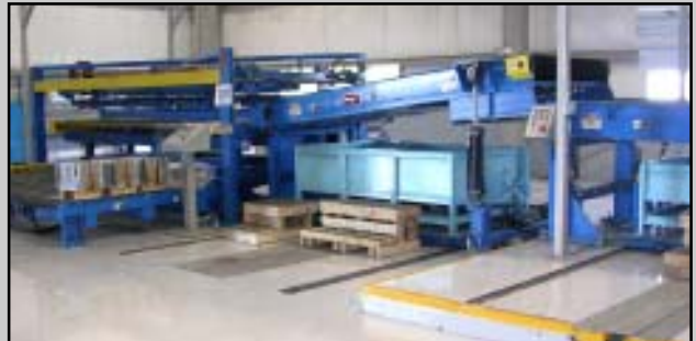
Variable Speed AC Motor Driven Belt Conveyor with Pop-Up Reject Mode
