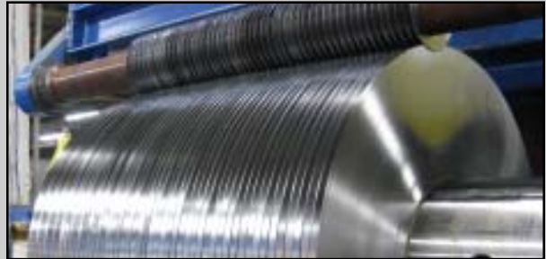
Winding 50-cuts 5/8" wide x .007" into tight perfect slit coils
