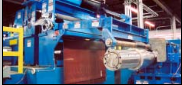
Recoiler produces 16" and 20" ID coils with or without cardboard cores
