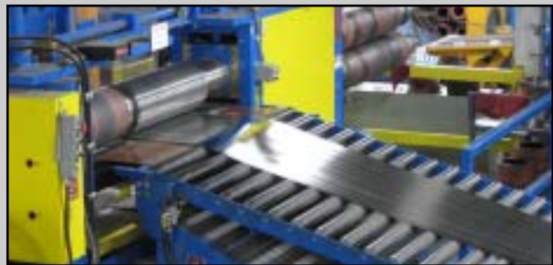
Turret Head™ Slitters offer quick tooling set-up, quick head change, and precise knife clearances
