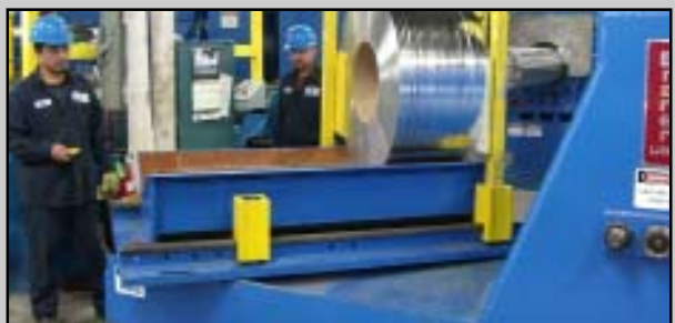
Rotary Deck Coil Car with Wireless Control
