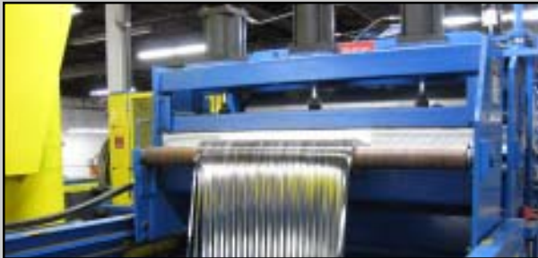
Thin gauge narrow strips guided into the Tensioners
