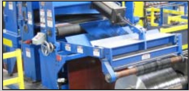
Close coupled Pass Line Roll provides excellent strip tracking to the Recoiler.
