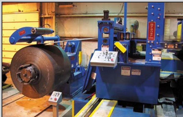
The Compact High Pass Line design processes coils without bending the strip against the natural coil-set. The Uncoiler is installed tight against the Entry Unit, which minimizes coil threading time and conserves floor space.
