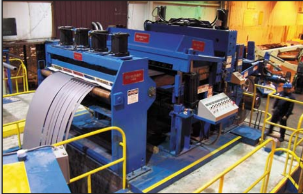
The Exit End equipment generates strip tension, crops coil tails, and rigidly supports the Overarm Separator
