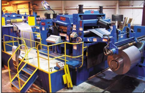
60,000# x 72" x 1/4" Single-Loop Turret Head™ Slitting Line with a Shape Correction Cluster Leveler™ that corrects edge-wave, center-buckle, and cross-bow strip shape defects.
