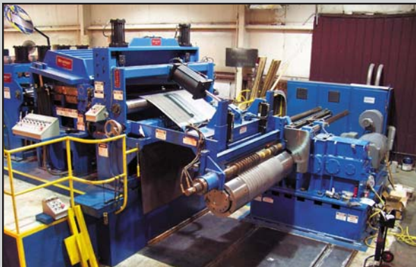
The Cluster Leveler™ is installed between the Tensioner and the Exit Shear. With its seven (7) adjustable back-up flights and work roll bend capability, the Cluster Leveler™ does not depend on tension for shape correction, and therefore will not "neck" the strip and reduce slit width dimensions.
