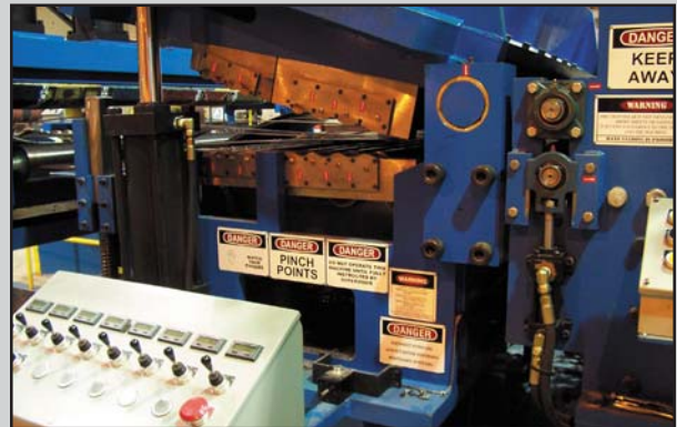
Specifically designed for coil-to-coil applications, the Cluster Leveler™ employs non-driven work rolls. The hydraulic cylinder "quick-open" feature allows coil threading to be quickly accomplished.
