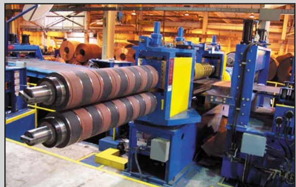
Turret Head™ Slitters are precise and rugged, and offer bullet-proof reliability. Head change time is less than two-minutes.
