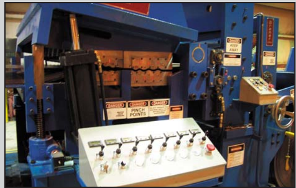
The Cluster Leveler™ employs its large work roll cluster to shape correct .150" gauge x 50,000 PSI pickled & oiled coil. The Cluster Leveler™ is a unique patented roller leveler designed specifically for coil-to-coil shape correction applications where the range of coil gauge and yield strength parameters far exceed CTL line gauge and strength capacities. Joy stick controls allow the operator to override the PLC automatic set-up and make roll bend adjustments while running.
