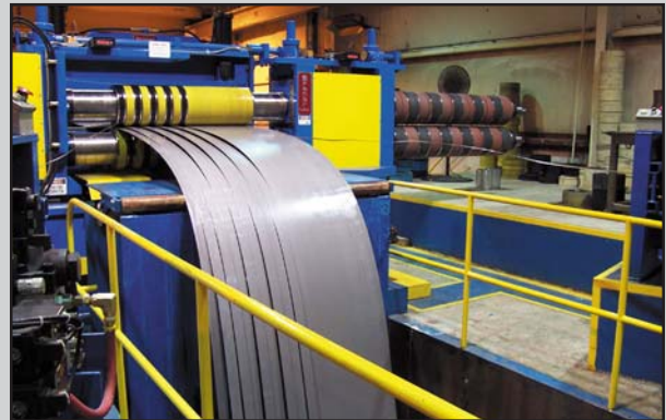
Turret Head™ Slitters are precise and rugged, and offer bullet-proof reliability. Head change time is less than two-minutes.
