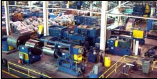
60,000# x 72” x .250”/.019” Hi-Performance Cassette Leveler-Servo-Feed-DC Shear CTL/Multi-Blank Line
