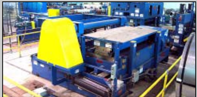
1.500” x 17-Roll x 7-Adjustable Flight x 5-Hi Cassette Produces Laser Quality Flat Strip
