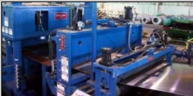
60,000# x 72” x .250”/.019” Hi-Performance Cassette Leveler-Servo-Feed-DC Shear CTL/Multi-Blank Line
