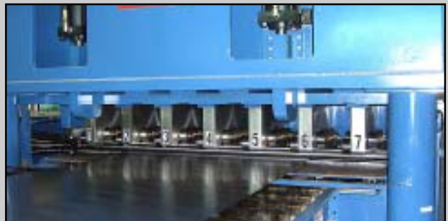
1.500” x 17-Roll x 7-Adjustable Flight x 5-Hi Cassette Produces Laser Quality Flat Strip
