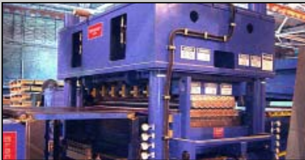
3' x 5-Hi Cassette installed in the 4-Post Leveler frame
