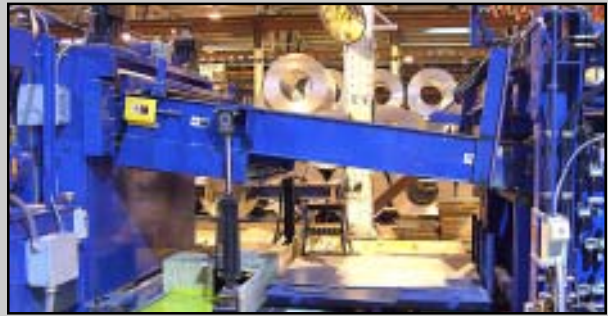
Inspection/Reject Conveyor carries sheets to the Stacker or diverts to a Scrap Cart
