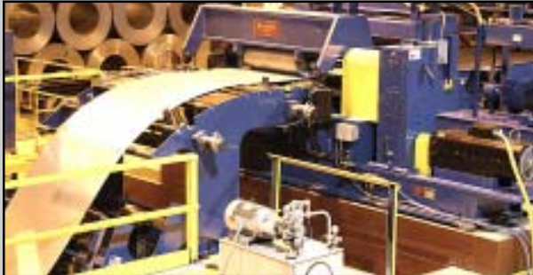
Hi-Performance Electronic AC Servo-Feed features a high cyclic rate and a "pull-back" sequence that avoids Shear blade scuffing.
