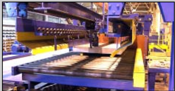
Automatic Sheet Stacker produces solid block sheet packs.
