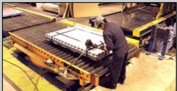
Automatic Sheet Stacker produces solid block sheet packs.
