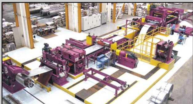
60,000# x 72” x 135% .028” Hi-Performance Cassette Leveler-Servo-Feed-DC Shear CTL/Multi-Blank Line
