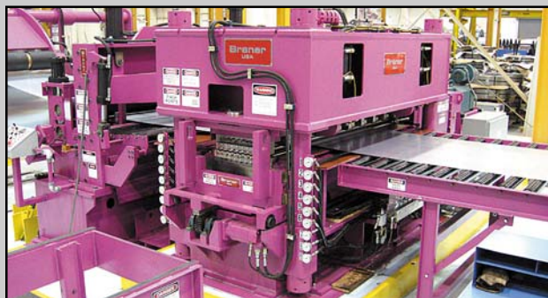
All Metals’ Hydraulic Cassette Leveler Produces Laser Quality Panel-Flat Strip. Cassettes can be power exchanged in a matter of minutes.
