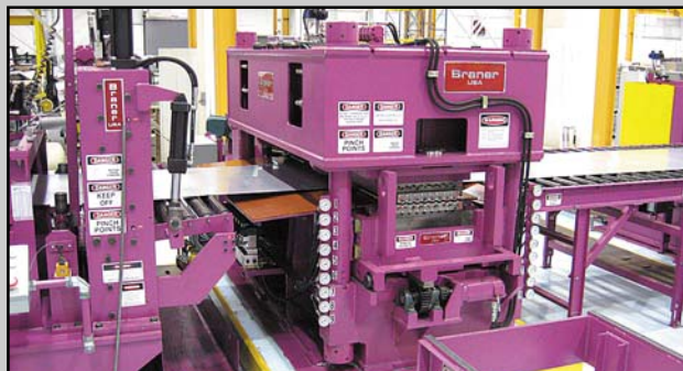
Precision Microprocessor Controlled Hydraulic Cassette Leveler Operating with 1.750” x 5-Hi Cassette
