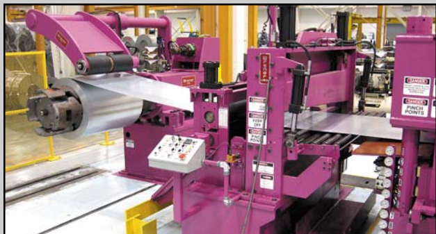
60,000# x 72” x 135% .028” Hi-Performance Cassette Leveler-Servo-Feed-DC Shear CTL/Multi-Blank Line
