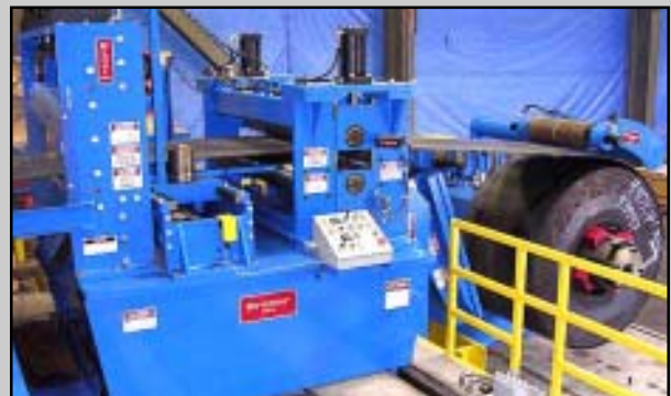
The Compact High Pass Line arrangement processes coils without bending the strip against the natural coil-set. The Uncoiler and Recoiler are installed tight against the entry and exit stations, reducing coil threading time and conserving floor space.
