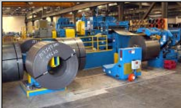
Four Arm Turnstiles stage and store 80" diameter coils at the entry and exit ends of Searing's 1/2" Slitting Line.
