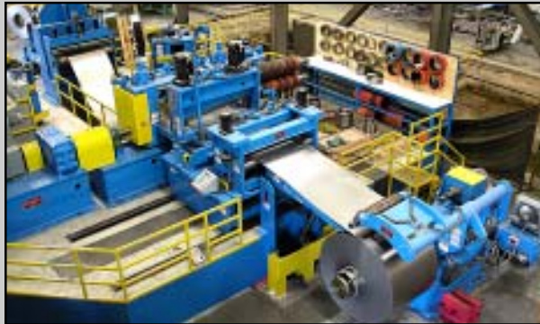
Single-Loop Turret Head™ Slitting Line processes hot rolled and cold rolled carbon steel coils in gauges from .060" through 1/2" in tight-line and single-loop operating modes.
