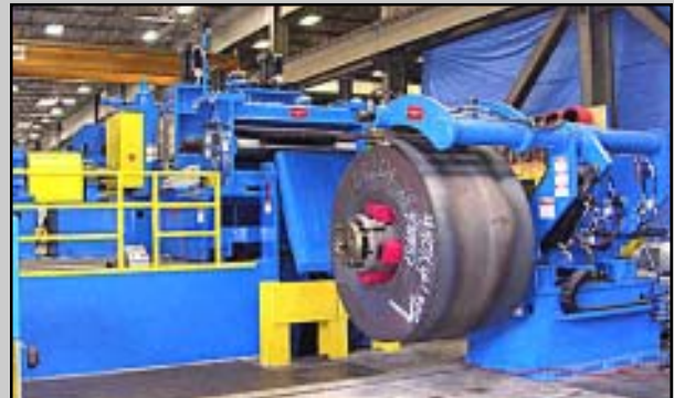
The Compact High Pass Line arrangement processes coils without bending the strip against the natural coil-set. The Uncoiler and Recoiler are installed tight against the entry and exit stations, reducing coil threading time and conserving floor space.
