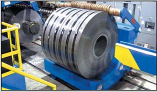
Sit coils are removed from the Recoiler and transferred to a 4-Arm Turnstile via Coil Car. The Car is equipped with an Overarm Hold-Down that stabilizes narrow coils during transport. Wireless radio controls eliminate electric cable maintenance and allows the operator to keep a safe distance away from the coil and Coil Car when operating.
