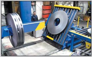
Slit coils are removed from the 4-Arm Turnstile and positioned onto power conveyor by an "Operatorless" Programmable Downender. The operation of the Downender is fully automatic and operatorless after the slit coil width data is programmed into a PLC controller.
