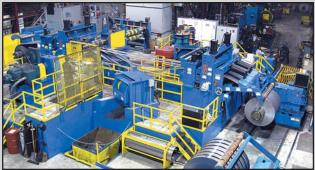
Single-Loop Turret Head<sup>™</sup> Slitting Line processes high-strength hot rolled and cold rolled carbon steel coils in gauges from .024" through 5/16" in tight-line, push-pull, and single-loop operating modes.
