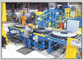
Coil strapping is quickly and easily accomplished on a semiautomatic Coiltech Strapping Machine. A pushbutton operated Power Coil Grab is employed for palletizing and coil stacking.
