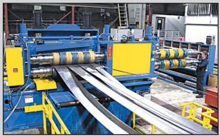
Turret Head<sup>™</sup> Slitters are rugged, precise, and are bullet-proof reliable. Head change time is less than two-minutes. Jennmar's "Pushbutton Tooling Lock-Up" allows re-tooling to be accomplished fast, and arbor/nut thread maintenance and repair is eliminated.
