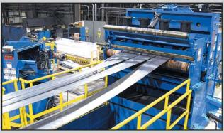
A pneumatic Pad Tensioner generates strip tension necessary to produce tight straight-wall slit coils. To reduce order change down-time, the tension pads can be exchanged in 60-seconds when the pad surface is worn, and the underarm separator arbor can be exchanged with a pre-tooled arbor in 30-seconds.
