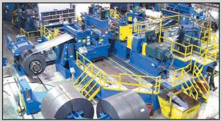
Jennmar's Turret Head<sup>™</sup> Slitting Line is equipped with Entry & Exit 4-Arm Turnstiles, Coil Straightener, Entry & Exit Shears, and 700 line horsepower.
