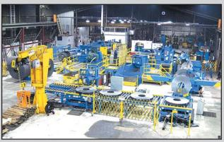
Slit coils generated by Jennmar's Turret Head<sup>™</sup> Slitting Line are quickly and efficiently packaged on a Compact Packaging System. The System has the capacity to handle 10,000# coils from 1" to 24" wide.
