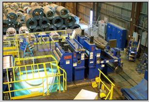
Strip tension required to generate tight straight-wall slit coils is generated by a Pad Tensioner and a Non-Marking Roll Tensioner. The Pad Tensioner is employed when slitting noncritical coil, and the Roll Tensioner is utilized for processing surface critical coated carbon steel, aluminum, and stainless coil. The Pad and Roll Tensioners can be engaged independently or in tandem. An Exit End Shear squares coil tails and eliminates the need to re-thread the line when splitting coil ODs.
