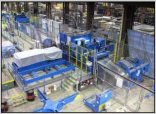
Russel Metals' Cassette Leveler CTL Line is capable of processing an extremely wide product and gauge range. Master coils are staged on an Entry 4-Arm, where a floor level Car transports and loads coils onto the Uncoiler. An Entry Coil Flattener straightens and threads the coil into the Entry Shear where the head end is cropped-off and collected in a Power Scrap Cart.
