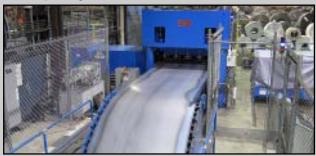
Russel Metals' CTL operates in a "free-loop" Servo Feed mode when processing 1/4" and thinner gauges, and runs in a stop-start mode when processing heavy gauge where a 1,000 PIW coil contains between 500 and 1,000 feet of material. A stable free-loop is maintained during the feed/shear cycle by a non-contact sonic sensor installed halfway along the loop length.
