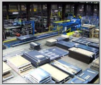
Top-quality panel-flat sheets of 1/2" hot rolled, bare and coated cold rolled carbon steel; plus aluminum and stainless with and without laminated PVC and paper interleaving, assembled into straight-sided packages is the product of Russel Metals' new Cassette Leveler/Servo Feed CTL Line.
