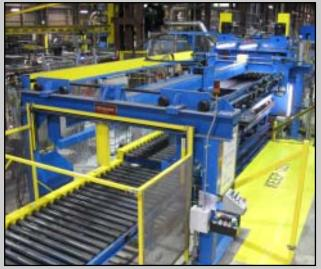
Straight-sided sheet packs are produced by the Automatic Sheet Stacker that efficiently handles surface-critical coated steel, aluminum, and stainless sheets without surface damage. The Stacker is able to stack sheets onto pallets or runners.
