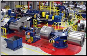
SteelSummit's latest high-performance slitting line employs 600 horsepower for processing surface-critical automotive coils weighing 70,000# in widths to 76" at slitting speeds to 1,000 FPM. Coil gauge capacity is from .012" minimum through .187".
