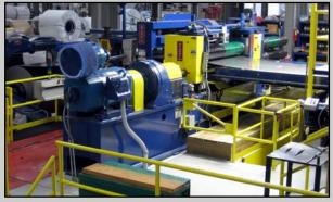
SteelSummit's Turret Head<sup>™</sup> Slitter produces close-tolerance slit strips with minimum burr throughout the entire range of
