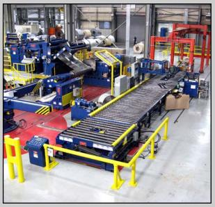
Slit coils are quickly and efficiently packaged for shipment on a Slit Coil Packaging Line capable of handling 10,000# coils in widths from 1" through 24". An "Operatorless" Programmable Downender automatically retrieves coils from the 4-Arm Turnstile and deposits them onto a conveyor line. Coils are quickly radially strapped and forwarded to the stacking station where the slit coils are palletized and packaged for shipment.
