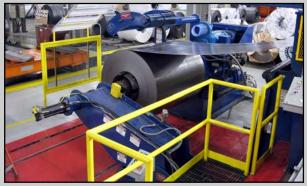
The DC motor driven loop-control Uncoiler fitted with an Outboard Support drives the coil into a free-loop ahead of the slitter in the Double-Loop tension-free slitting mode. Tensionfree slitting eliminates tooling induced strip surface scuffing, and generates tighter tolerance slit widths. Single-Loop and two (2) Tight-Line operating modes are employed for slitting medium and heavier gauge coil.
