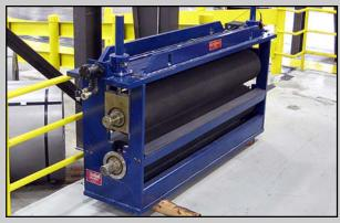
In order to maintain exceptional surface-critical quality standards, SteelSummit's Non-Marking Tensioner is equipped with quick-change tension roll cartridges that are employed for dedicated critical quality products
