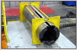
The Slitting Line can produce slit coils with 20" and 24" IDs. A patented Speed-Load Filler allows SteelSummit to change coil IDs in 2-minutes, a task that requires 15-20 minutes with older technology "bolt-on" style filler plates.
