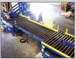
Slit coils generated from the Turret Head™ Slitting Line are quickly and efficiently strapped and packaged for shipment on a Slit Coil Packaging Line capable of handling from 1" through 16" wide coils. An "Operatorless" Programmable Downender automatically retrieves coils from the Turnstile and deposits them onto a conveyor line. Slit coils are efficiently strapped and transported to a stacking station where coils are palletized and wrapped for shipment.
