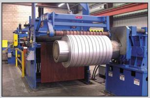
Globe Stainless' Recoiler is equipped with a 20" diameter rewind drum powered by a large DC motor driving through a parallel shaft helical gear reducer. A swing-out quick-change Overarm Separator is firmly supported from the Exit Unit to assure the Overarm tooling is square and parallel with the Recoiler when running. Pre-tooled Overarm arbors can be exchanged in about 2-minutes.
