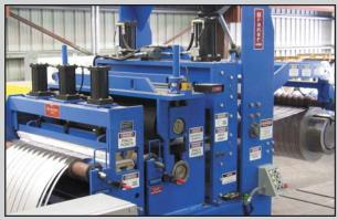
Strip tension necessary to produce tight straight-wall slit coils is generated by a Pad Tensioner and a Non-Marking Roll Tensioner.. The Pad Tensioner is engaged when slitting noncritical surface coil, and the Roll Tensioner is employed when processing bright and polished finish stainless coil. The Pad and Roll Tensioners can be engaged independently or in tandem. A guillotine Exit End Shear squares coil tails and eliminates the need to re-thread the line when splitting coils.
