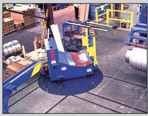
A floor level Coil Car with "wireless" operator controls quickly unloads slit coils from the Recoiler and transports the coils to a Turnstile and Packaging Line. A power Turntable rotates the Coil Car 90-degrees to line-up with the Pack Line.
