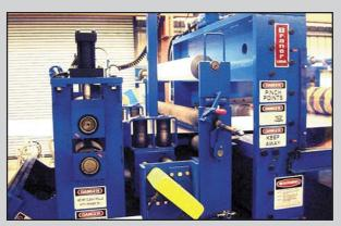
A floor level Coil Car with a "wireless" operator control loads coils onto the Uncoiler. Paper interleaved between coil wraps
