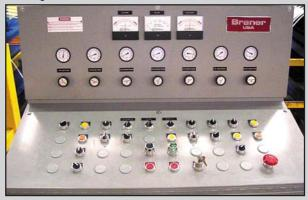
The main operator console is ergonomically designed to make operating the Slitting Line efficient and safe. Clear sight lines allow the operator to view the entire line without cameras and TV monitors.
