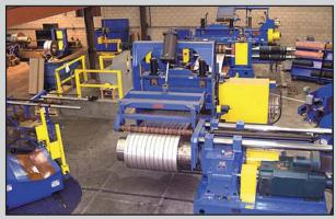
Globe Stainless' high-performance slitting line has the capacity to efficiently convert 60" wide 300 and 400 series stainless steel coil in all finishes into precise width straight-wall PVC laminated or paper interleaved slit coil.. Gauge capacity is from .015" minimum through .187". A single-loop mode or either of two (2) tight-line operating modes can be employed, depending upon coil specs and slitting load.
