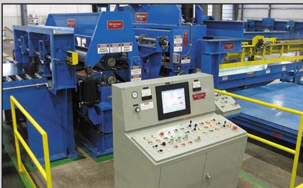
Cascadia's CTL Line features Braner/Loopco's fast and reliable Hi-Speed Hydraulic Shear. Adjustable blade gap allows Cascadia to quickly and easily establish the ideal blade clearance for shearing carbon steel and aluminum alloy throughout the .028" to .250" gauge range. Notable benefits of the Hi-Speed Hydraulic Shear are its exceptional reliability and virtual noise-less shearing cycle.
