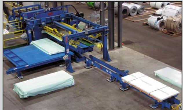
A finished sheet pack awaits removal while a new pack is being generated in the Stacker. A fresh skid placed on the Injector Table awaits injection into the Stacker.
