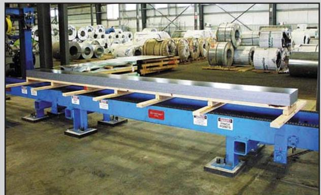
Panel-flat 14-gauge x 14,500" wide x 180" long sheets stacked in straight-sided solid block sheet packs.
