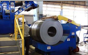
The 60,000# Recoiler, powered by a 250 HP motor and a two-ratio parallel shaft helical gear reducer, can produce 20" and 24" ID coils. A patented "Speed-Load Filler" gives American Strip the ability to change from 20" to 24" ID coils in one-minute rather than the 15-20 minutes required to install common "bolt-on" style fillers. Slit coils are unloaded from the Recoiler and transferred to the Pack Line Turnstile via Coil Car fitted with a pushbutton engaged narrow coil stabilizer.
