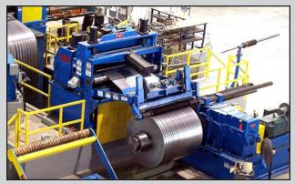
A Pneumatic Pad Tensioner that generates winding tension necessary to produce tight straight-wall slit coils is installed on the Exit Unit. Quick-change pads and underarm separator can be exchanged in less than one-minute. An Exit Shear, Tail Feed Rolls, Pass Line/Tach Roll, Overarm Separator, Recoiler Feed Table, and safety Coil Tail Hold-Down are installed on the compact Exit Unit.
