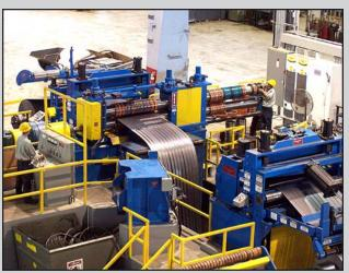
The quick-change precision Turret Head™ Slitter produces close-tolerance slit strips with minimum burr throughout the entire range of gauge and mechanical properties. The unique unobstructed open arbor Turret Head™ Slitter design speeds re-tooling and accomplishes a head a change cycle in one-minute. Reliability is bullet-proof.
