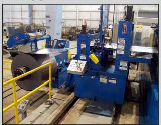
Quick coil threading, superior strip tracking, elimination of equipment induced coil-breaks, and excellent operator sight lines are among the many benefits of the compact high pass line equipment arrangement. Entry and Exit Turnstiles, Entry and Exit Shears, laser beam coil alignment, fiber optic automatic servo edge guiding, plus many other performance features enhance American Strip's ability to efficiently process small and large orders throughout a gauge range from .015" through 1/4".
