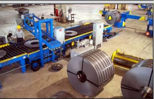
Slit coils are efficiently packaged for shipment on a Slit Coil Packaging Line capable of handling 15,000# coils in widths from 1" through 24". An "Operatorless" Programmable Downender automatically retrieves coils from the 4-Arm Turnstile and deposits coils one at a time onto a conveyor line. Radial straps are quickly applied by a semi-automatic Slit Coil Strapper, and the strapped coils are conveyed to the Stacking Station where slit coils are palletized and prepared for shipment.
