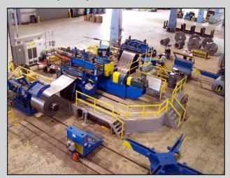
American Strip's latest high-performance slitting line processes 60,000# x 72" hot rolled, cold rolled, and galvanized coils at speeds to 1,000 FPM. Coil gauge capacity is from .015" through .250". Single-Loop or either of two (2) Tight-Line slitting modes can be employed for processing a wide range of gauges and mechanical properties.
