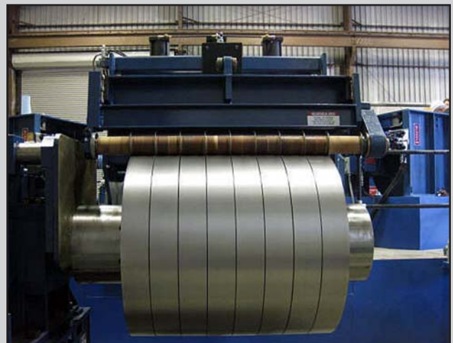
A high-torque 2-ratio Recoiler is equipped with a massive Recoiler drum manufactured from custom forged 2” thick segments hardened to Rc 58. A 3” diameter solid steel gripper bar grips slit strips against a heat-treated serrated steel anvil. The Recoiler drum is installed on the 14” diameter output shaft of a 1.2 service factor parallel shaft helical gear reducer. The result is the production of superb quality slit coils.
