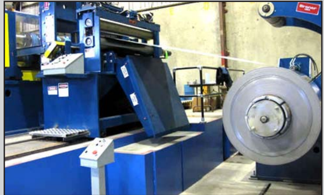
The Compact Hi Pass Line arrangement allows quick threading, elimination of induced coil-breaks, provides superb strip tracking, and reduces the line length to 37-feet.
