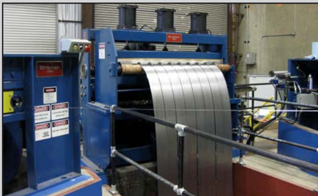
Multiple strips are precisely guided from the free-loop into a Tension Stand that generates high strip tension for producing tightly wound straight-wall slit coils.
