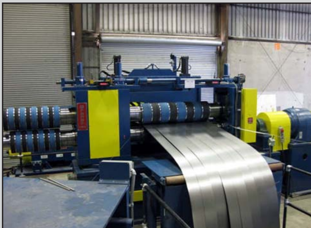
40,000# x 60" x .135"/.024" Single-Loop Turret Head™ Slitting Line at California Steel & Tube
