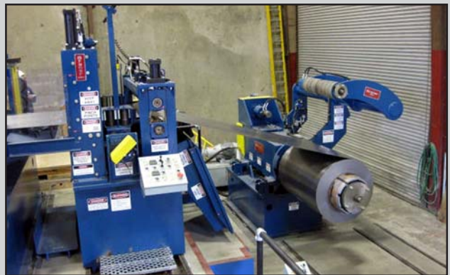
Entry Station combines entry coil threading and guiding equipment into a single compact machine that speeds coil threading and improves strip tracking.
