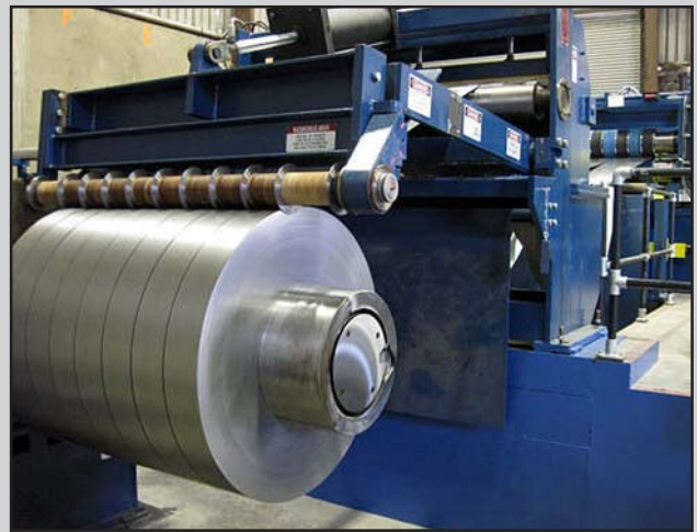
Overarm frame deflection and misalignment that results in coil side-wall scuffing and coil oscillation is eliminated by rigidly mounting the Overarm onto the Exit Unit housing. A quick-change “swing-out” Overarm arbor allows pre-tooled arbors to be exchanged in 2-minutes when changing to the next order. A Hydraulic Threading Funnel directs slit strips from the Exit Pass Line Roll into the Recoiler gripper bar during threading.
